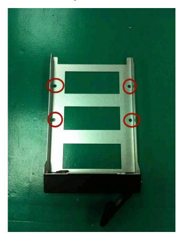
Once the tray is removed from the unit, notice there are four holes, which are used to secure the HDD.
